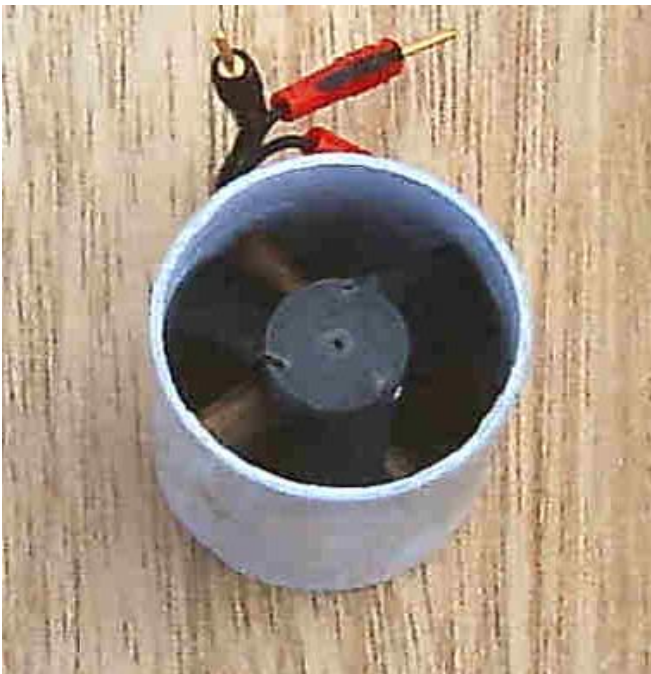
Top: Derek Knight's well-campaigned 13" span Swift has a new lease of life as an EDF test bed. It looks better than ever though it now weighs 80g. Note the sophisticated charger. Middle: LiPo battery installation with ESC controller. Bottom: Derek's 24 mm EDF unit. The tiny 10mm x 15mm motor is well-ventilated and can run at 65,000 rpm for up to two minutes at a time.
