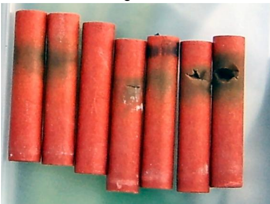
Above: a selection of the new red L2 motors ‘post-flight’. Note various degrees of scorching of the casing.
