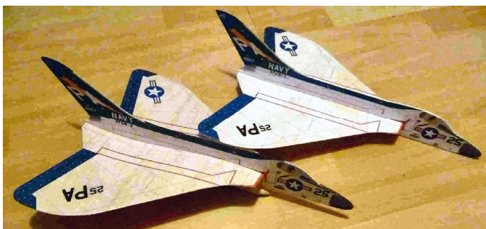
Above: Howard Metcalfe's contrasting Skyray (left) and 'Flatray'; Both are based on Bill Dean's originals; the Flatray, as the name implies, features a straight, not reflexed 'ogee' section, with elevons with 3° of 'up'. Both fly well, but differently.
