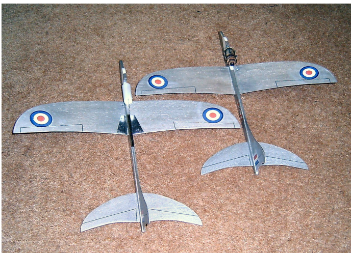
Above: Recreations of Mike Ingram's 1953 Sharky. Not quite 'ARTF' by today's standards, the die cut balsa sheets were unpainted; those for the fuselage needed laminating and the wings had to be cemented together before slotting in. Kits were otherwise complete with cement, motor, asbestos sheet, fuel, wick, and those distinctive decals.
